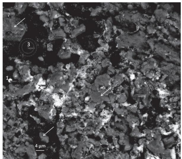
Fig. 5. SEM-BSE (scanning electron microscope-backscattered electrons) images of the cell wall of charophyte cell exposed to 100 mg/l nCuO for 3 h. Dark regions represent “clean” cell wall surface not covered by calcium carbonate deposits. The bright spots are CuO nanoparticle aggregates. On the right picture, the numbers show spots where elemental analysis, an EDX (energy dispersive X-ray system), coupled to the SEM was accomplished. Arrows show calcium carbonate deposits
