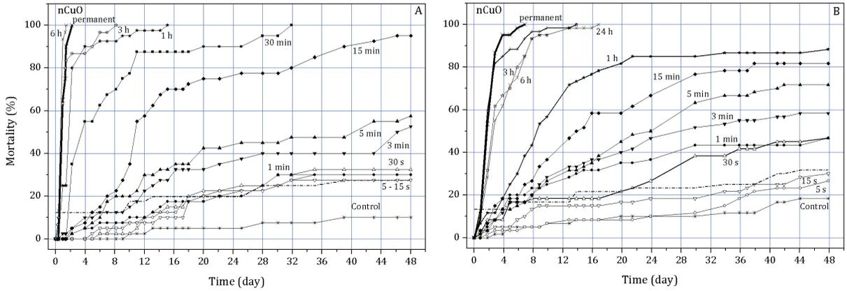
Fig. 2. Mortality kinetics of charophyte algae cells of *Nitellopsis obtusa* in control medium after exposure for 5 s–24 h to 79.9 (A) or 24 mg Cu/l (B) in nCuO suspensions. Thickened lines represent permanent exposure in corresponding medium. Dash dot lines represent statistically significant difference from controls at  $\alpha = 0.05$ ;  $n = 40$  and  $60$  cells/treatment, respectively (A) and (B)
