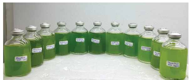
Fig. 1. Microalgae cultivation in 60 ml sealed sterile vial serum bottle for hydrogen production
