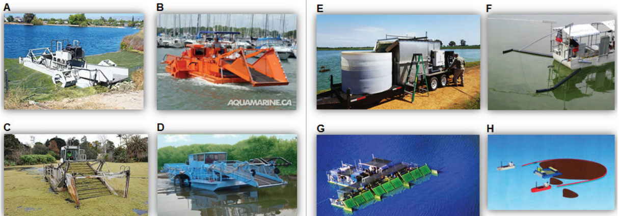
Fig. 1. The examples of manufactured harvesters for collection of aquatic vegetation and macroalgae (A–D) or cyanobacteria scums in small water bodies (E–F) and large water ecosystems (G–H). A – Harvester for aquatic vegetation and algae (San Jose, California, USA). https://commons.wikimedia.org/wiki/File:Algae_harvester-2.jpg [Accessed on 20-05-2019]; B – H5-200 Aquatic weed harvester Aquamarine H5-200 (Ontario, Canada). www.aquamarine.ca/aquatic-weed-harvesters/ [Accessed on 20-05-2019]; C – Azolla harvester (India). www.azollaamrit.com/gallery.php?pid=6 [Accessed on 20-05-2019]; D – SINOBE-ACON Automatic Underwater Aquatic Vegetation cutting device (China). 803768290/Specially_Designed_Automatic_Underwater_Aquatic_Vegetation_Harvester_For_Sale.html [Accessed on 20-05-2019]; E – ALGENT – mobile cyanobacteria harvesting platform (USA). www.smithsonianmag.com/innovation/startup-harvesting-wild-algae-make-your-next-pair-sneakers-180960872/ [Accessed on 20-05-2019]; F – ASIO – vessel for cyanobacteria harvesting (Czech Republic) www.asio.cz/en/vessel-for-the-separation-of-biomass-particles [Accessed on 20-05-2019]; G – Aphanizomenon flos-aquae scum harvester from Lake Klamath (USA). https://cerulequebecfr.com/tag/algue-klamath/ [Accessed on 20-05-2019]; H – modified oil boom for harvesting cyanobacteria scums in the Baltic Sea, Sweden (GRÖNDAHL, 2009)
